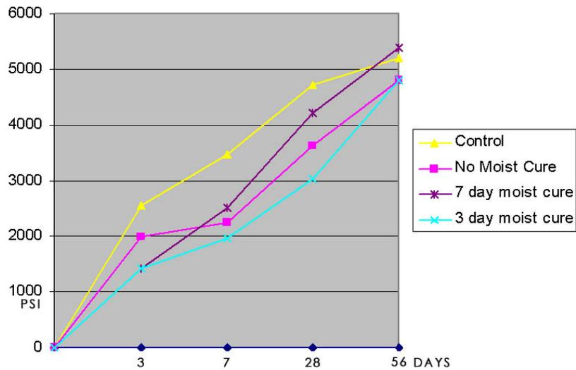
**Figure 4: Core data – Strength vs. Age**
