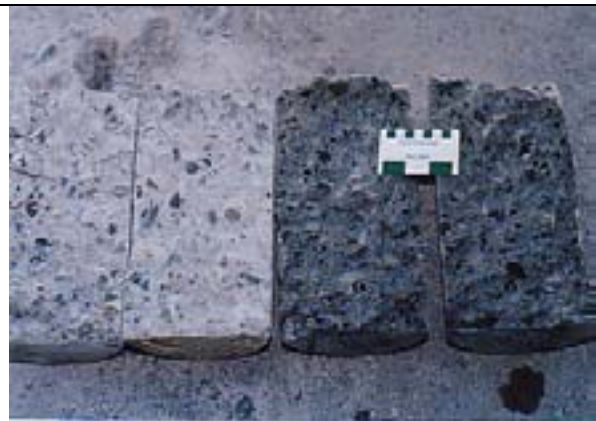
Photograph 8 Split tensile test cylinders after testing. Right = Wet. Left = Dry.
