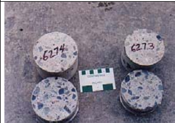
Photograph 7 Cylinders prepared for Phase I RCP test. Lower faces polished. #6273 is Test Mix; #6274 is Supplementary Mix.
