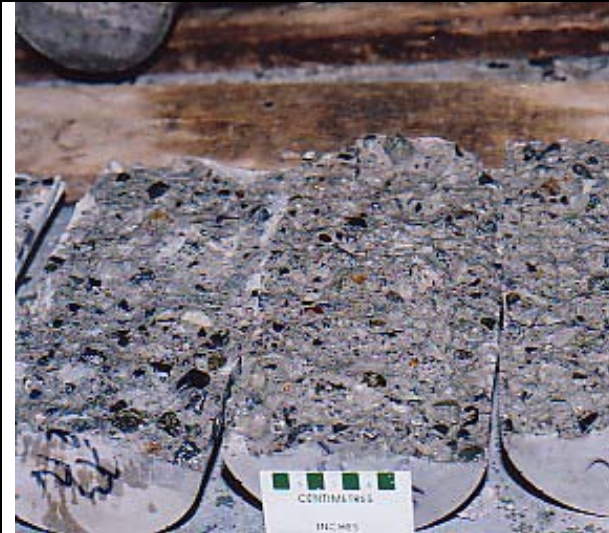
Photograph 9 Close-up of Photograph 8. Note some coarse aggregate fractured but most failed in paste:aggregate bond.
