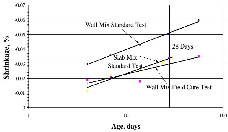
**Fig.7. Shrinkage Vs Time (Test Batch)**
