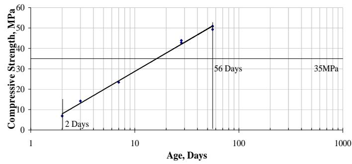
**Fig.6. Wall Concrete – Age: Strength Relationship**
