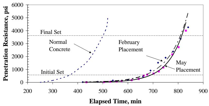
**Fig.5. Setting Time for Wall Concrete – Winter vs. Spring**
