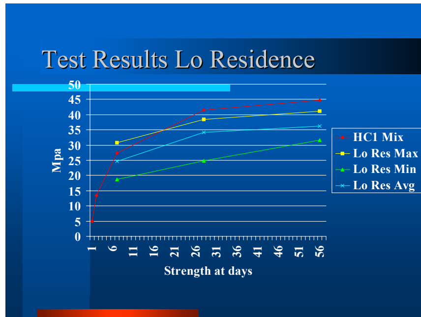
Figure 3: Test Results of Lo Residence HVFA Mix as Compared to HC1 Mix
