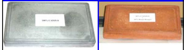
Figure 25 100% Alkali-activated glass frit mortar
