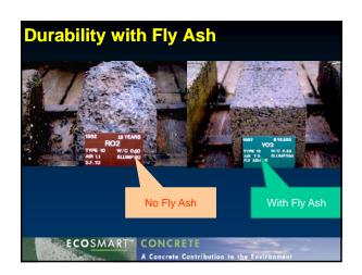
Fly ash makes concrete easier to pump and place and reduces the heat of hydration
