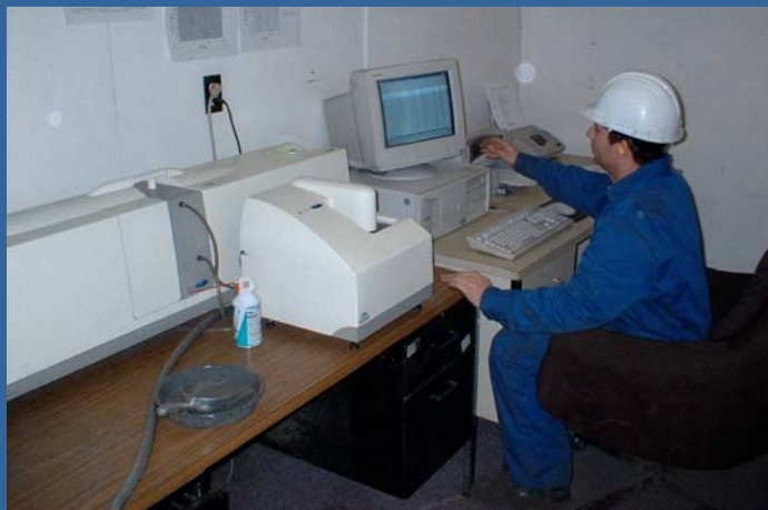
Malvern Laser Particle Size Analyzer for Quality Control
