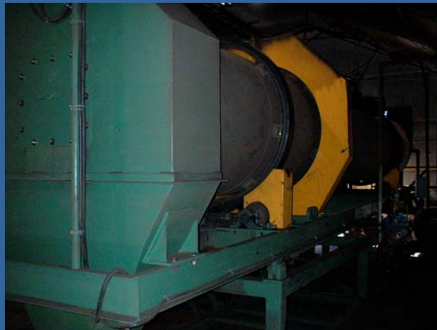
Natural Gas Fired Rotary Dryer
