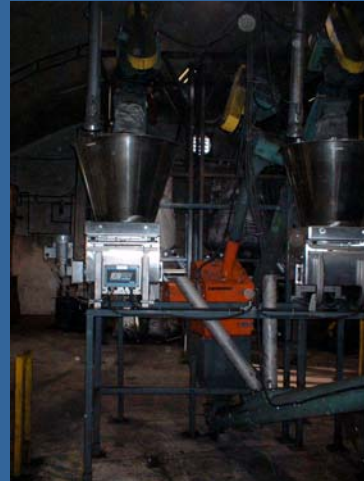
Computerized Proportioning of Ingredients Prior to Intergrinding
